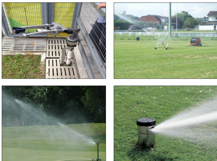
Fig. 3. Types of irrigation systems used in the sports turf industry. From left to right: canon type, self-travelling type, static type and pop-up type. Only automatic pop-up irrigation systems are considered appropriate for pitches used to host UEFA matches
