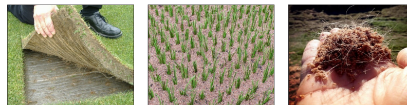
Fig. 5. Types of turf reinforcement system. From left to right: carpet, stitched and fibre
