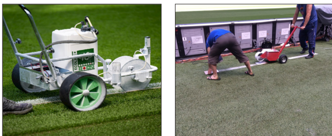
Fig. 18 Wheel-to-wheel line marking following a string line (left) and marking out dashed lines (right)
