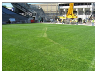
Fig. 84. Cool-season turf that has suffered minimal damage from light-duty protective panels left in place for six days.
